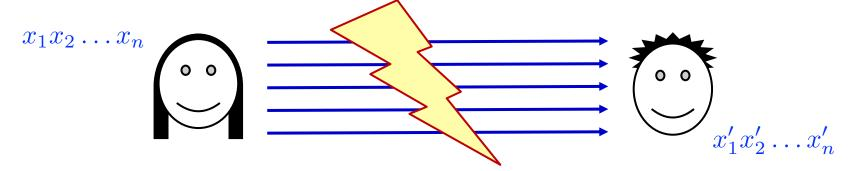
One simple noise model is the *binary symmetric channel*, where each bit flips with probability  $\varepsilon$  (independently)
