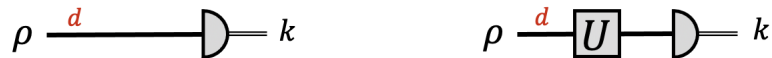
Figure 13: Measurement with respect to the computational basis and a basis specified by U .
