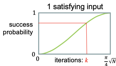
Figure 19: Success probability of measurement as a function of k , the number of iterations.
