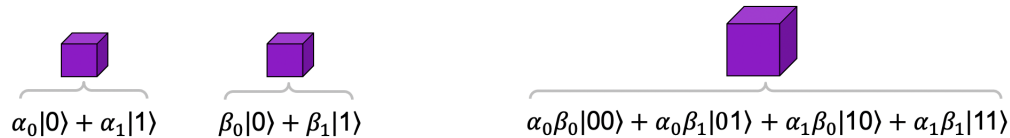
Figure 31: Two separate qubit state vectors can be translated into a 2-qubit state vector.
