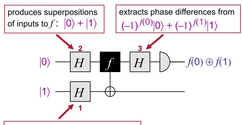
constructs eigenvector so *f*-queries induce phases:  $|x\rangle \rightarrow (-1)^{f(x)}|x\rangle$
